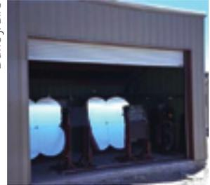
*This figure shows the kind of detector at HiRes Fly's Eye. UV light caused by an air shower's excitation of atoms is reflected by mirrors into a box containing hundreds of photomultiplier tubes. A picture of this air shower can be reconstructed from the time of the light's arrival and the amount of light collected by each tube. This technique works on clear, moonless nights, using very fast camera elements to record light flashes just few microseconds in duration.*
