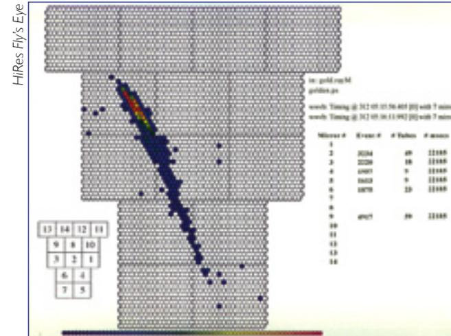
*This is an actual readout from the HiRes detector. Each hexagon represents a photomultiplier tube. Colored hexagons represent photomultiplier tubes that have detected UV light. The elongated image represents the actual shape of the air shower.*
